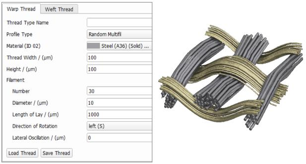
**Filament - Diameter** determines the diameter of the filaments in a multifilament thread.
