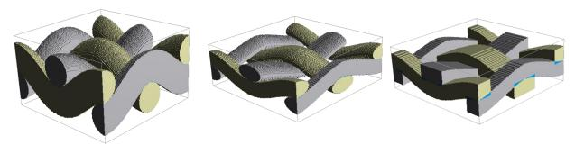
For all profile types, **Material** designates the Material assigned to the thread. **Width** and **Height** determine the cross-section area of the thread. For the **Monofil Circular** profile type, only the **Width** can be entered.
