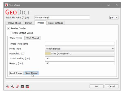
Different threads might overlap in the generated structure. This might be unintuitive, but it leads to realistic thread shapes at contact points. Therefore, the thread overlap allows to create realistic weave structures without the need for simulating the physical effect of the thread contacts.
