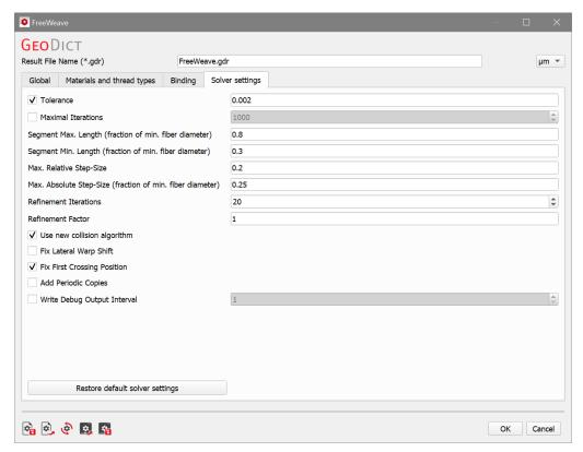
At the beginning of the **Solver** run, the fibers are subdivided into smaller segments over several iterations given by **Refinement Iterations**, which are part of the solver iterations. This is also the minimum number of iterations. Other stopping criteria are only considered when the **Refinement Iterations** are exceeded.
