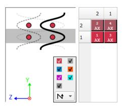
The preview of the **Weft-Layer System** shows all weft layers in vertical direction. The first layer is in the first column from the right. Each layer is displayed in a 2D preview and a table.
