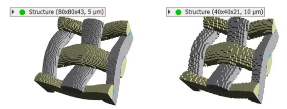
The values entered for **Inflow Region** and **Outflow Region** determine the size of the void regions below (-Z direction) and above (+Z direction) the generated woven structure.
