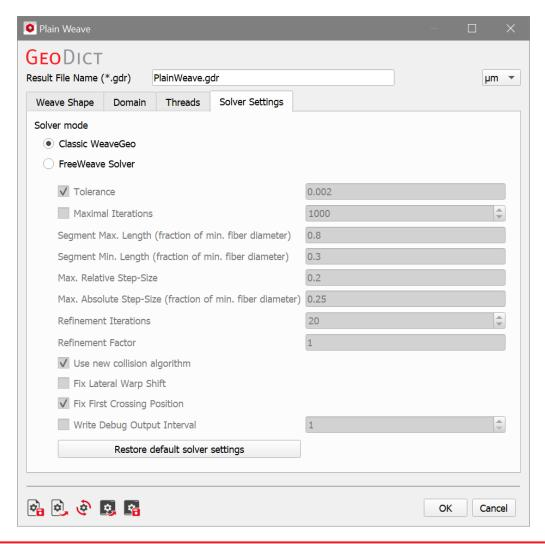
The parameters entered in most GeoDict dialogs, here especially in the Plain Weave, Twill Weave, Satin Weave, or Free Weave dialogs can be saved into \*.gps (GeoDict Project Settings) files and/or loaded from them. Remember to restore and reset your (or GeoDict's) default values through the icons at the bottom of the dialog when needed and/or before every WeaveGeo run.
