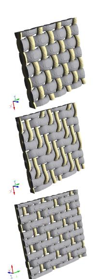
The **Plain** weave is the simplest weave type. Each weft is alternately placed above and below a warp thread, creating the characteristic cross (or checkerboard) pattern. Each unit cell contains two warp and two weft threads.
