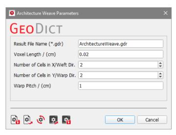
By clicking the **Options' Edit...** button, the corresponding parameter dialog is opened and the main parameters defining the weave can be changed.
