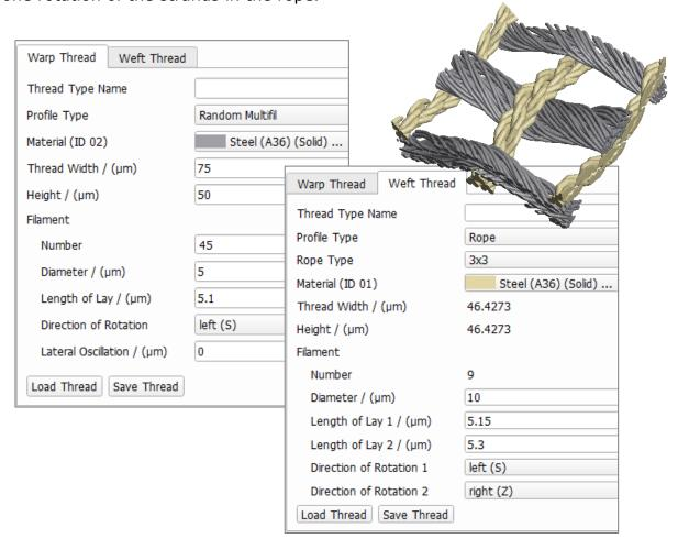
**Direction of Rotation 2** controls the direction of rotation of the strands: **right** (Z-twist strand) or **left** (S-twist strand).
