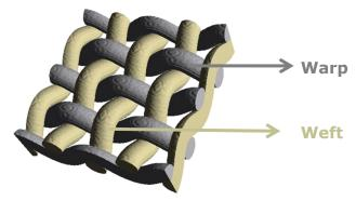
Different settings can be chosen for the warp and weft threads. Here below, a **Monofil** elliptical thread has been selected for the **warp** (and different width and height entered) whereas the **weft** is a **Monofil** circular thread.
