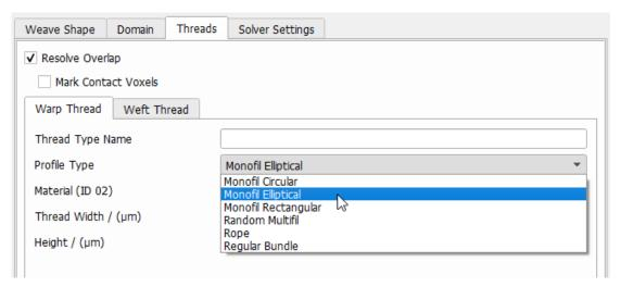
Refer to page <u>6</u> for explanations on **Monofil**, **Multifil**, **Rope**, and **Regular Bundle** profile types. **Monofil** threads can have a **Circular**, **Elliptical**, or **Rectangular** cross-section.
