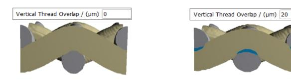
The **Crimp Factor** defines the straightness of the warp and weft threads. It varies between -1 and 1. A value of 1 for the **Crimp Factor** results in straight weft threads, while a value of -1 results in straight warp threads. When it is set to 0, both thread types bent around each other, leading to a thinner structure. With the **Crimp Factor**, all possible gradations between the extremes Dutch Weave and Reverse Dutch Weave can be achieved.
