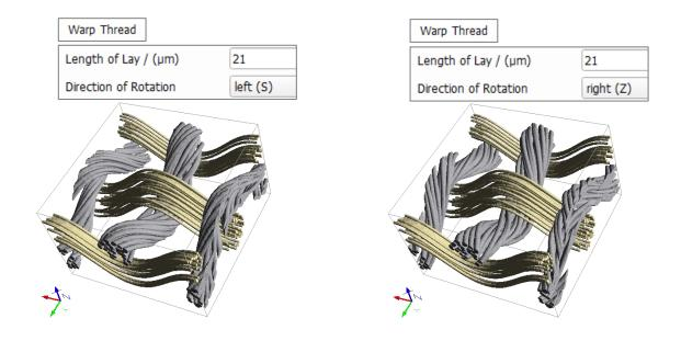
For ropes with several strands (here the **weft** thread), the **Length of Lay 1** is the length for one rotation of the rope (thread) and **Length of Lay 2** is the length for one rotation of the strands in the rope.
