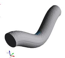
A thread which is composed of many filaments is called **Multifilament** or **Multifil** thread. For multifilament threads it is necessary to model the position of the center of the filament profiles in the threads, and the geometry of the filaments.
