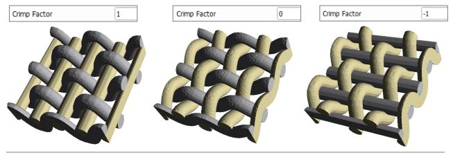
**Warp** and **Weft Broadening** are the relative spreading of the threads at the interlacing points of weft and warp threads. This spreading simulates the bending and deformation of the threads during the weaving process. Values of broadening vary between 0 (no broadening) and 1.
