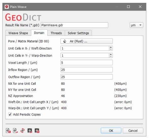
The **Voxel Length** is the size of a voxel in the chosen units. To see the difference that the increase in voxel length produces, select the **Box renderer** under **View** → **3D Structure Renderer** → **Box**, and not the **Smooth** renderer (since this option softens the visualization).
