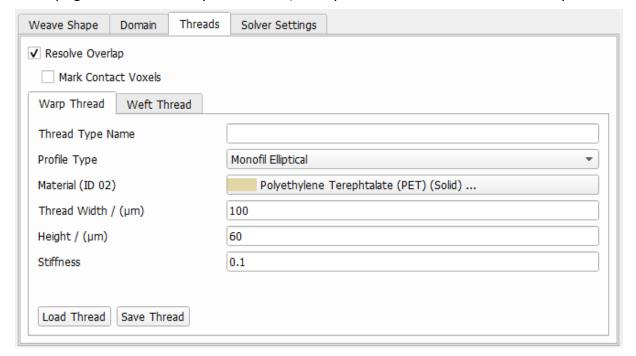
A high **Stiffness** indicates a rigid thread that only bends in small angles. Values for Stiffness can vary from 0 to 1.
