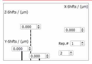
If two warp or weft threads overlap, they are marked with a yellow sign with exclamation mark in the preview of the **Warp-Layer System**. The overlap is not checked in z-direction. This initial overlap can be resolved by either adjusting the binding or using **Shifts**.
