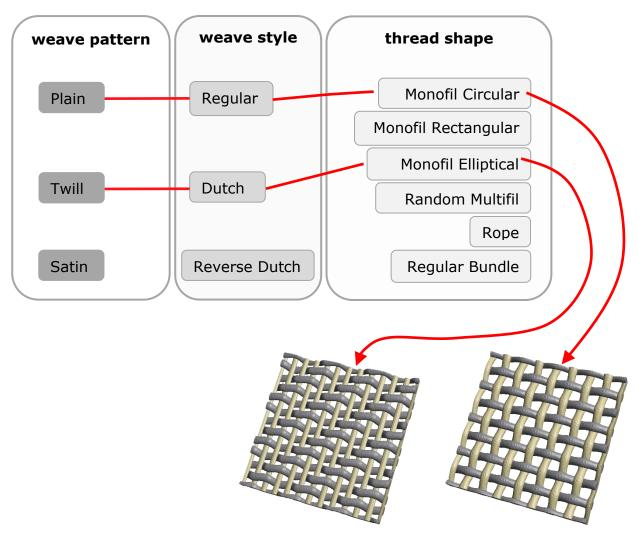
The choice of weave type (and material) determines the final properties of the woven structure, such as weight, wettability, stability, flexibility, porosity, or smoothness.
