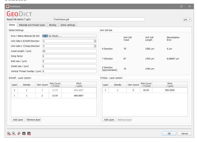
The values in **Unit Cells in X/Weft-Direction** and **Unit Cells in Y/Warp-Direction** set the number of repetitions of the generated unit cell. For periodic simulations, one unit cell is sufficient.
