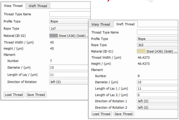
**Length of Lay** is the distance in which the thread (and its filaments) is rotated 360° around its axis. The **Length of Lay** must be chosen so that the unit cell is periodic. In other words: The unit cell length must be a multiple of the **Length of Lay**. Otherwise, a warning message appears, and the parameter is adjusted automatically. The choice of unrealistically short values might lead to artifacts in the generation and, therefore, to unrealistic structures.
