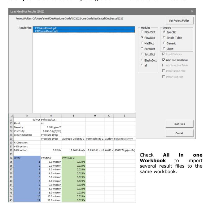
After the general and the geometry information, the user gets access to data on the pressure drop, the average velocity, the permeability, the Gurley value, the flow resistivity, the flow rate etc. and to the pressure per layer, in all computed directions.
