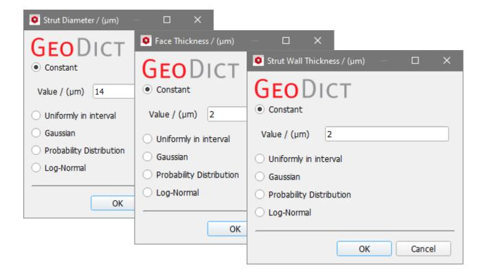
Observe the effect of entering values of **Strut Diameter**, as shown in the dialog boxes, on the generated random foam shown on the right.
