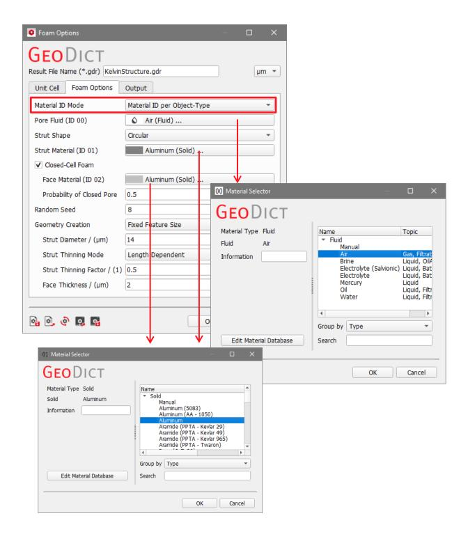
For **Material ID Mode** Material ID per Material, Strut Material and Face Material are assigned to the same Material ID (ID 01), if the same material is chosen.
