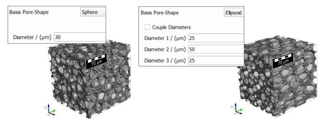
As explained in pages <u>8ff.</u> for strut diameters, the diameter of the spheres (**Diameter**) or ellipsoids (**Diameter 1** in X-direction, **Diameter 2** in Y-direction, **Diameter 3** in Z-direction) can be changed by clicking **Edit...**.
