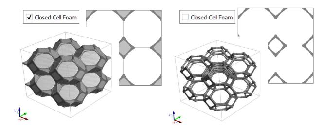
When the structure is a closed-cell foam, values between 0 and 1 can be entered for the **Probability of Closed Pore**. When the value is 1, all pore walls are closed. When the value is 0, the result is an open foam.
