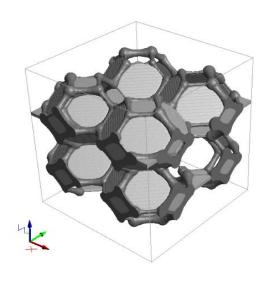
Taking the **Gaussian** (or **normal**) distribution, the value follows a bell-shaped distribution. The strut diameter value clusters around the entered **Mean Value** but may vary according to the entered **Standard Deviation**.
