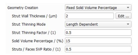
For both modes, the thinning of struts is defined by the **Strut Thinning Factor** and the **Strut Thinning Mode**. The **Strut Thinning Factor** determines the rate by which the diameter of the strut diminishes toward the center of each strut. The **Strut Thinning Mode** defines if this thinning depends on the length of the strut or is independent on the length.
