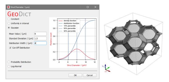
If **Cut-Off Distribution** is checked, the distribution is truncated at the bounds. This means, that all values outside the bounds are dropped and not considered for generation. If this option is not checked, then all values that are outside of the bounds are set to be on the distribution bound.
