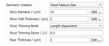
**Strut Diameter** distribution and **Face Thickness** distribution can be entered by checking the **Edit...** buttons in this mode.
