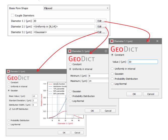
When **Ellipsoid** is the Basis Pore-Shape, a probability can be assigned to the combination of the three diameters by checking **Couple Diameters**. Instead of independent probability distributions for diameter 1, for diameter 2 and for diameter 3, the three coupled diameters share the same probability in the distribution.
