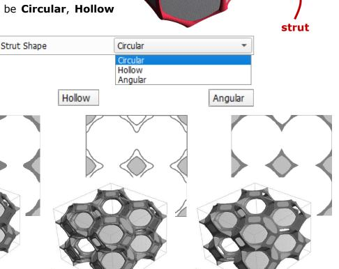
For the **Material ID Mode** Material ID per Object-Type, the fluid in the pore space (Pore Fluid (ID 00)), and the solid material for the **Strut Material (ID 01)** and, below, the **Face Material (ID 02)** can be selected from the Material Selector by clicking the buttons consecutively.
