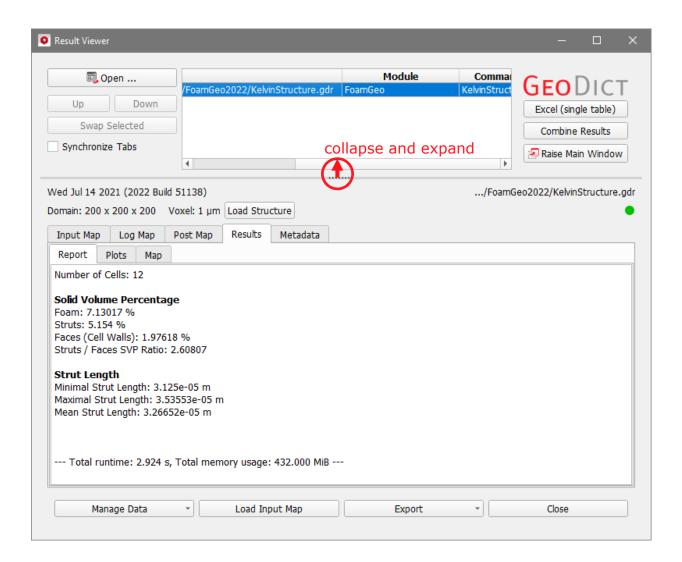
On the **Results** tab, the subtab **Report** lists the solid volume percentages (SVP) for the whole foam, as well as for struts and faces separately. The Struts / Faces SVP Ratio is the SVP of the struts divided by the SVP of faces, here 5.154 % / 1.976 % = 2.608.
