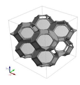
When selecting **Uniformly in interval**, and entering a **Minimum** value and a **Maximum** value, the strut diameter can take any value within this interval.
