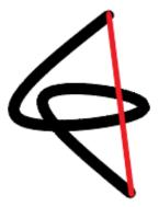
FiberFind extracts the centerlines of fibers via skeletonization and calculates the curvature and curliness based on the centerline and the length of fibers. If no analytic data (.gad) is available, e.g., from a previously run fiber identification, FiberFind identifies the fibers with the classical image processing approach first.
