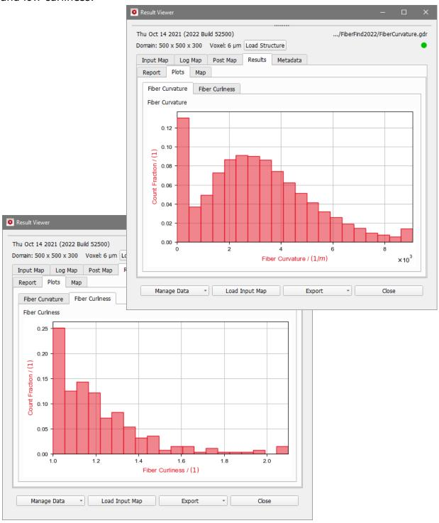
Besides analyzing the fiber curvature in the structure, FiberFind creates a model of the structure by extracting all fibers of the structure and creating fitting analytic fiber models if no analytic data was available for the structure before.
