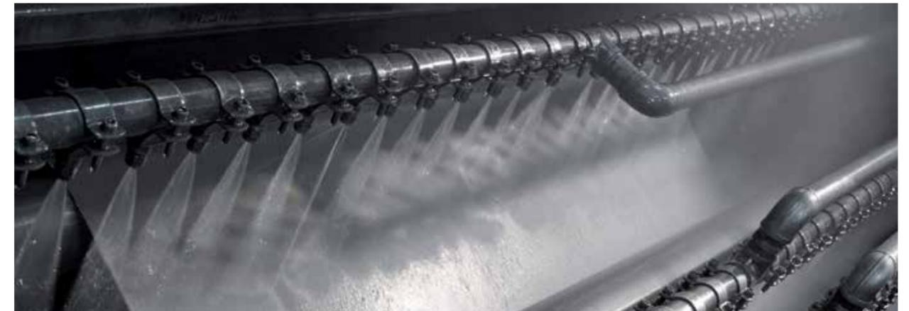
To provide our premium sand screens without any signs of dirt is a necessity as well. Dirt, dust and oil might still remain on the surface of wires after the weaving process. Therefore GKD has several continuous cleaning devices in place which use the power of ultra-sonic.
