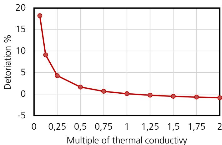
Figure 9: Deterioration on a percentage basis in comparison with the unplastered strip ceiling with 5 mm thick plaster system of various thermal conductivity as a multiple of the value of plaster system FH (0.49 W/(m<sup>2</sup> K)).
