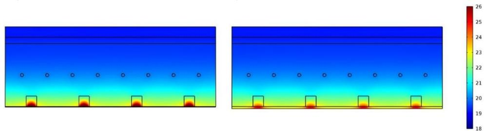
Figure 8: Distributions of simulated component temperature given in degrees Celsius after 156 hours (at noon). Plaster system FH with halved thermal conductivity and 2.5 mm layer thickness (left) as well as with doubled thermal conductivity and 10 mm layer thickness (right).
