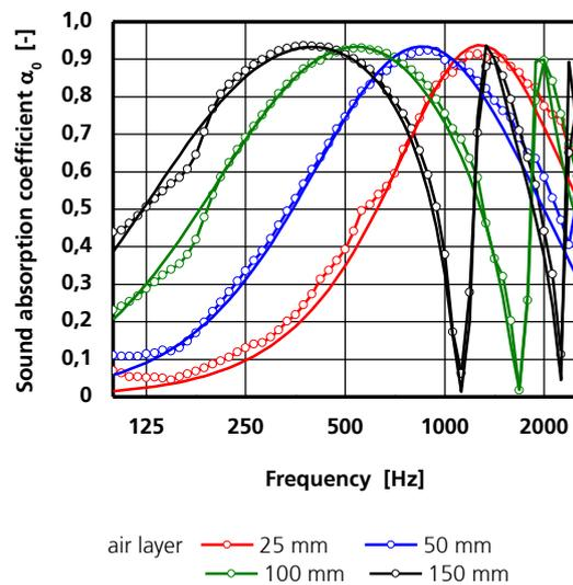
Figure 3: Comparison of the measured (dotted) and calculated (continuous lines) sound absorption coefficients of a sample of plaster FH in front of various air layers.
