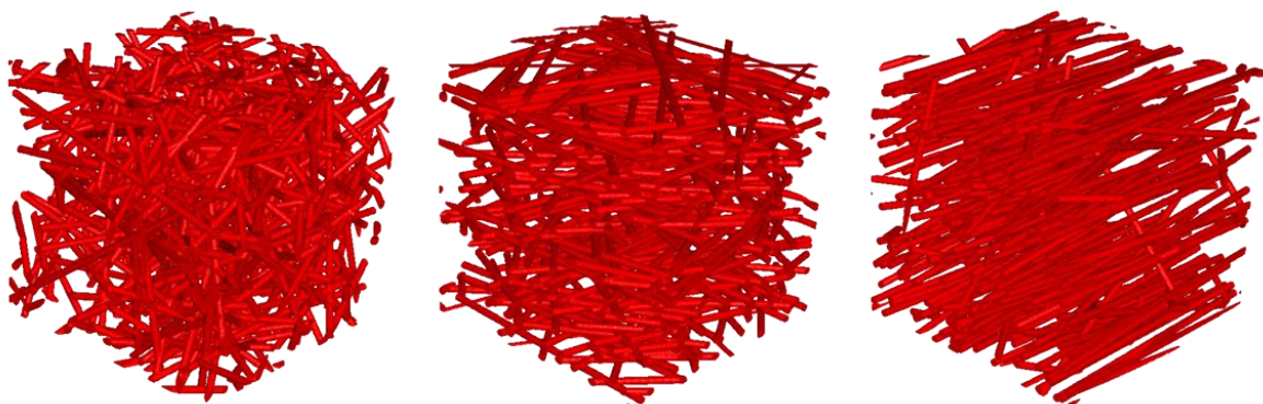
Fig 2. Structures with aligned fibers, planar randomness, and 3D randomness
