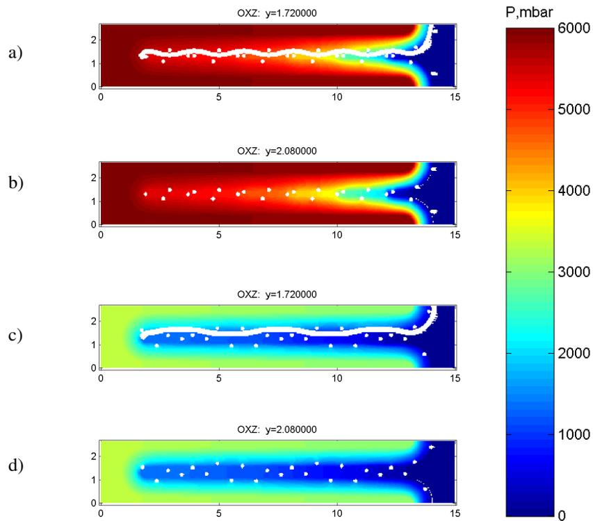
Fig. 4: a), b) show the pressure distribution ( $p + \int f$  in the notation from equation (5)) for the plain weave for two different cross sections. c), d) show the pressure distribution for the 2/2 twill for the same areas. White areas mark the solid wires. The filter media is not shown but it can be envisioned from the strong gradients in the pressure fields.
