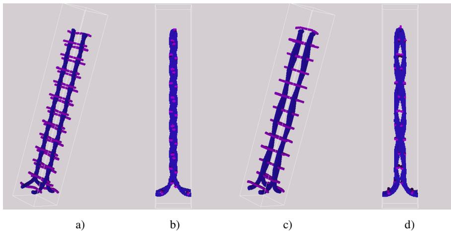
Fig. 3: The main difference between the original and the new design. The plain weave a), b) allows the blue wires to slide next to each other b) and creates a rather narrow outflow channel. For the same wire thicknesses, the 2/2 twill c), prevents the wires from sliding next to each other and creates a wider outflow channel d).
