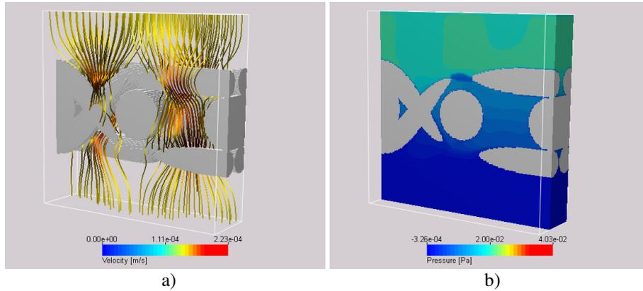
Figure 1: Stream lines (a) and pressure (b) for flow through a Dutch weave wire mesh computed via the Stokes equations. Computational box illustrated by its white edges.
