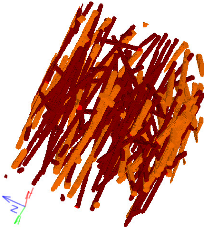
Figure 3. 3-dimensional view of a 200^3 realization of a nonwoven with two different fiber types. 5.4 dtex fibers are shown orange and 3 dtex fibers are shown in red. The anisotropic fiber orientation is “almost” parallel to the x-y plane.
