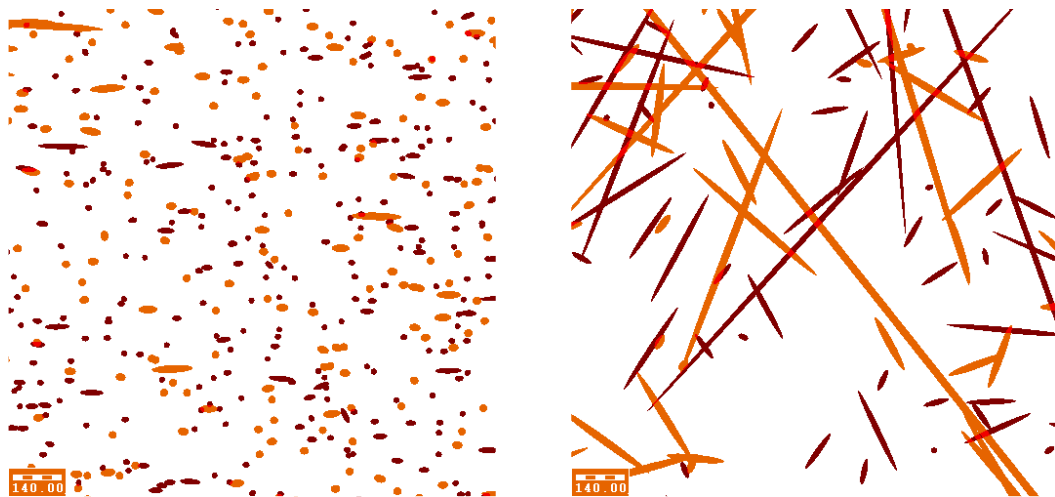
Figure 4. a) X cross section view of a 500^3 voxel virtual nonwoven media model with 90 % porosity. b) Z cross section view of the same, highly anisotropic media. The Y-cross section view looks similar to the X cross section view.
